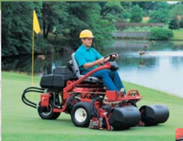
**ENVIED DESIGN** The legendary Toro triplex design, with its unique placement of the cutting units, offers numerous advantages, including the easy-empty center basket. Rear-wheel tracking within the radius of the front wheels helps keep operators out of trouble in sharp turns. The low-mounted engine and hydraulic components provide exceptional hillside stability. This configuration also improves service and maintenance accessibility.
