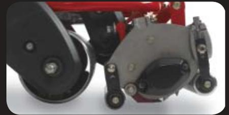
The cutting unit rollers are tucked closer to the reel and separated by a mere 8.25" (21 cm) to prevent scalping.
