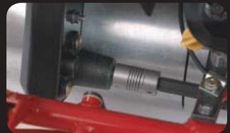
Flexible drive shaft couplers allow the cutting unit to flex on the center axis.
